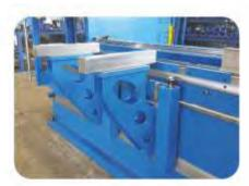
Heavy-duty front supports, moveable on linear guide, height adjustable (optional)
