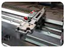
Automatic Thickness Measurement (ATM) and Bending Program Correction (optional)
