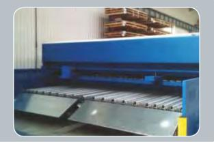
2-axis Back Gauge, X1-X2, for angle cutting
