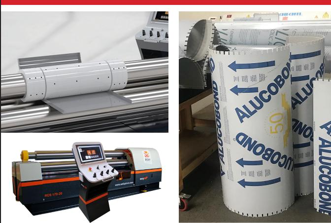
The Picot three-roll plate roll bending machines from Boschert USA deliver both the strength to form sheet metal and plate up to 39mm in thickness and 4100 mm in length *and* the dexterity to process the newest aluminum composite materials (ACMs) and three-dimensional parts, including plates with flanges. For powerful rolls with less flat edge pre-roll than 4-roll machines, and without damage to fragile ACM surfaces or structured 3D sheets, check out Picot.
