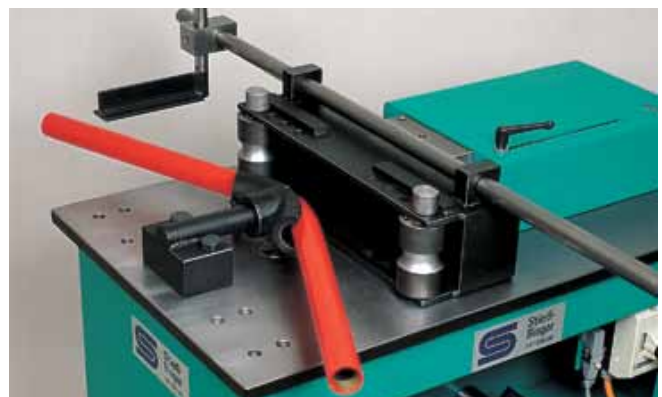
132 Gasrohrbiegen Bending of pipes
