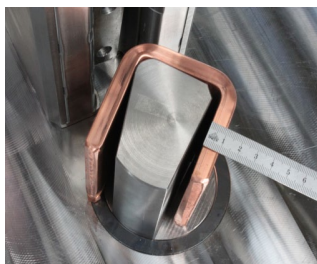
Narrow section punch, without support pin
