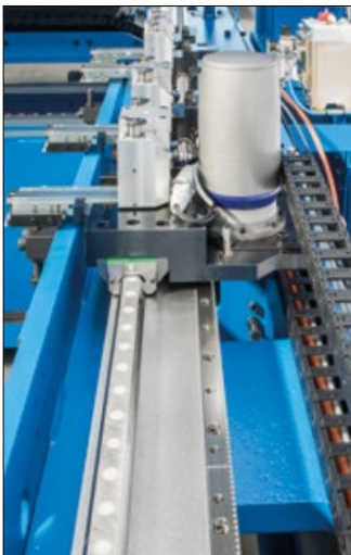
Servo geared motor with precision rack and pinion drive.
