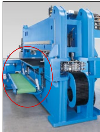
Solid welded steel construction guarantees the highest stability for punching sheets up to 12,7 mm thickness.
