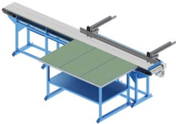
Unloading table with hinge conveyor and pusher
