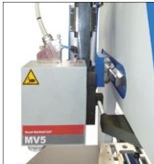
CUProfi and CuMaster marking unit: for labeling of finished parts
