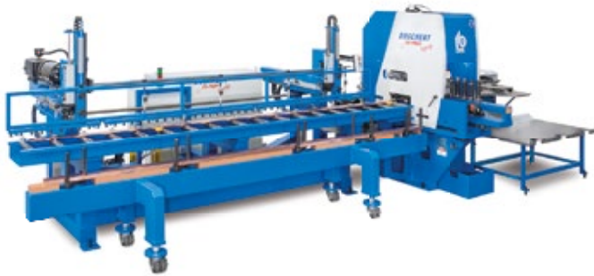
CUProfi and CuMaster loader. For automatic loading with pneumatic suction arms (4 oder 6 mm)
