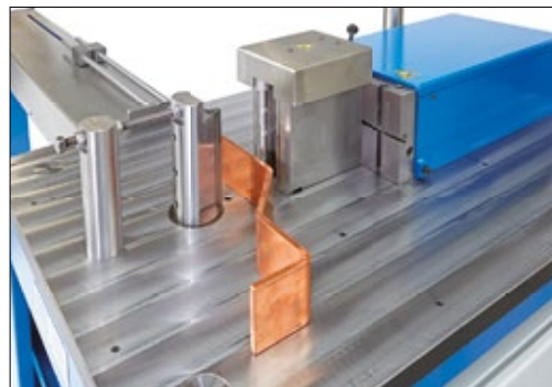
Measuring vee-block with automatic angle correction and bending without marks.
