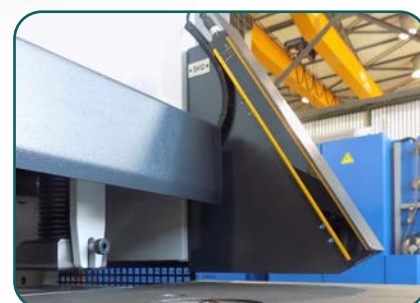
Finger protection with light guards (optional)
