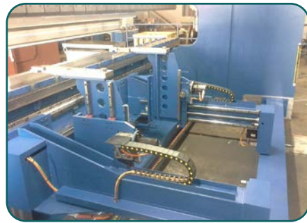
6-axis back gauge, X1-X2-R1-R2-Z1-Z2 (optional)
