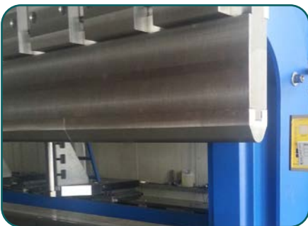
Heavy-duty clamping system up to 350t/m (optional)
