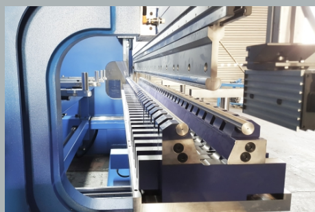
Special, heavy-duty, adjustable die, V=25 - 400mm.
