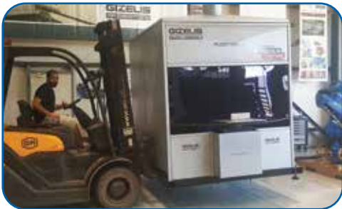
The compact cell can be repositioned quickly and easily using a forklift truck.
