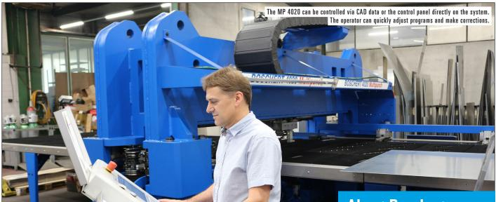
The MP 4020 can be controlled via CAD data or via the control panel directly on the system. Here the worker can quickly adjust programs and make corrections on a user-friendly interface.
