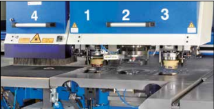
CombiCut laser TRI 3-head punching machine with 2xRevotool (head 1 + 3) and rotation / index (head 2)
