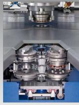
8 station tool carrousel with cassettes that hold punch, die and stripper or Revotool head with 4, 6 or 8 tools.
