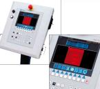
Control panel 10,5" TFT colour screen, ergonomically designed, it is adjustable and mounted on casters. USB, dual palm buttons, tool change position button, emergency-off. The powerful graphic and conversational software guarantees simple and fast programming. It is also available in a PC version.
