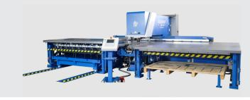
Punching. Forming. Marking. Fiber Laser Cutting. Boschert builds the broadest range of combination punch/laser machines in the world. Featuring working ranges from 30" x 80" to 60" x 120" plus repositioning. One, two or three punching heads or fully automatic tool changer. With full rotation, multi-tool, vertically moveable dies for deep forms and punching force to 50 tons.
